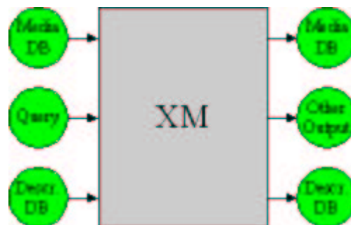
Figure 38: Interface model for XM key applications. This model shows the superset of possible inputs and outputs of an XM key application.
