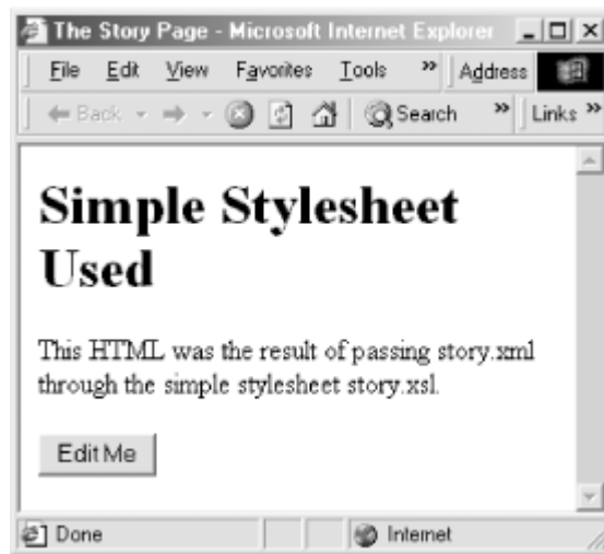
Figure 6-3. Transformation using a simple stylesheet
